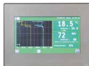
Controller a microprocessore touchscreen
